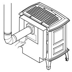
Figure 25 - Test for Proper Venting
